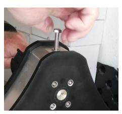
Lock the support shaft with the M8 x 90 screw
